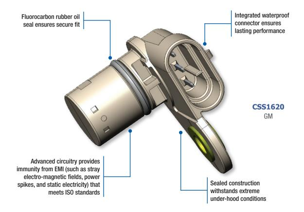
Tech Tip: To determine if a sensor is malfunctioning, use a scan tool to check the RPM while cranking the engine. If the engine runs, a scope is the best diagnostic tool.
