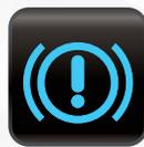
**Sistema de freno:** Indicates one of three possible conditions: parking brake is on; problem with the braking system/brake fluid is low, or ABS problem. Check brake fluid and make sure the parking brake is fully released. If the problem is in the ABS system, it may need a professional
