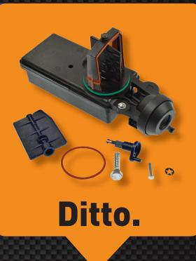
Over time, the OE flap on a DISA Valve becomes stripped, resulting in rough idle, loss of power and a DTC. Rather than replace the entire assembly, TechSmart® repair kits let you simply replace the damaged flap. It's the smarter, faster, and more economical repair – naturally.
