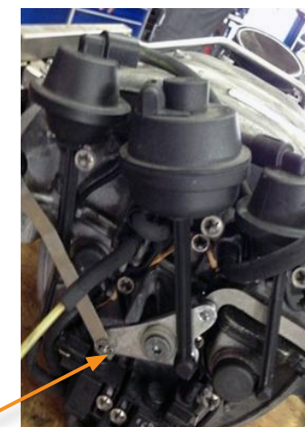
New TechSmart® unit installed on an old manifold
