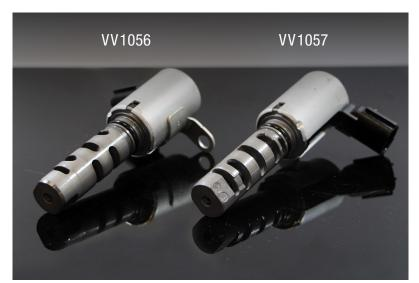
Years: 2001-2007 Make: Toyota Engines: 3.0L and 3.3L Common DTC: P1354 Symptoms: Rough idle Solution: Maintain regular engine oil change intervals. When replacing the solenoids, replace the engine oil and filter. Parts for the job: VV1056 and VV1057
