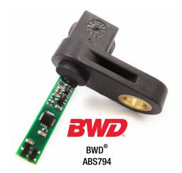
The BWD® ABS794 uses microsensors to produce the unique forward and reverse signals that modern vehicles require to keep electronic safety systems (Hill Hold Assist, ESC and Automated Braking) working correctly
